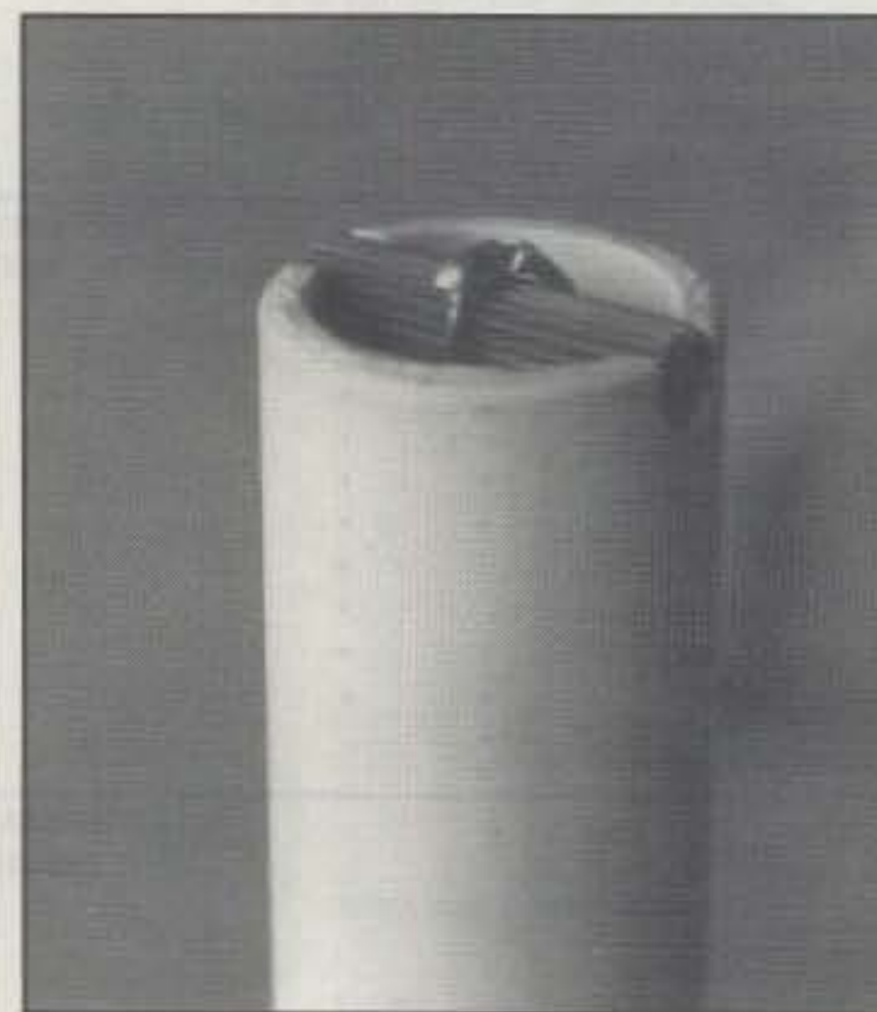
The top section of the antenna with the cap removed. You can see the loop of the antenna being supported by the \frac{3}{4} inch plastic rod, which rests in the cutouts.
