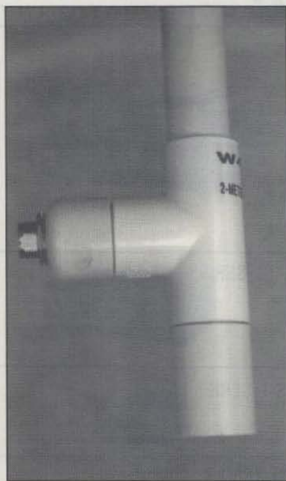
The bottom section of the antenna showing the SO-239 connector. At the bottom is a PVC coupling to facilitate mounting.
